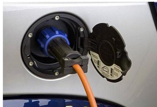
Figure 1 – Common plug used for charging an electric vehicle<sup>2</sup>
