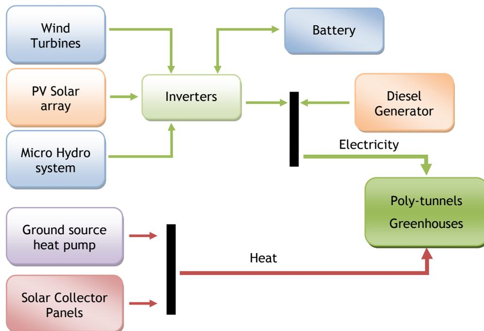
Figure 1. Schematic diagram of the Renewable Energy Croft
