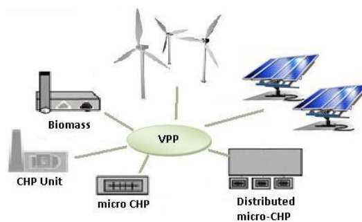
Figure 3 – Diagram for a Virtual Power Plant (VPP)
