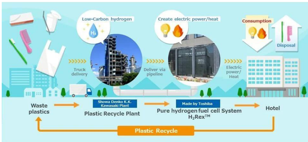
Figure 6.1 - Plastic recycling producing H 2 to supply heat and power to a hotel in Kawasaki
